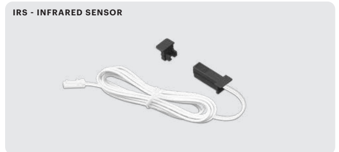
Proximity switch ON-OFF / DIMMER (10-100%) Range: 3-6cm
